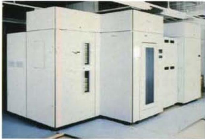
and transports. Each robot can access every cartridge and every tape drive in the library. Each is equipped with its own bar code label reader to clearly identify individual cartridges during mount operations.
